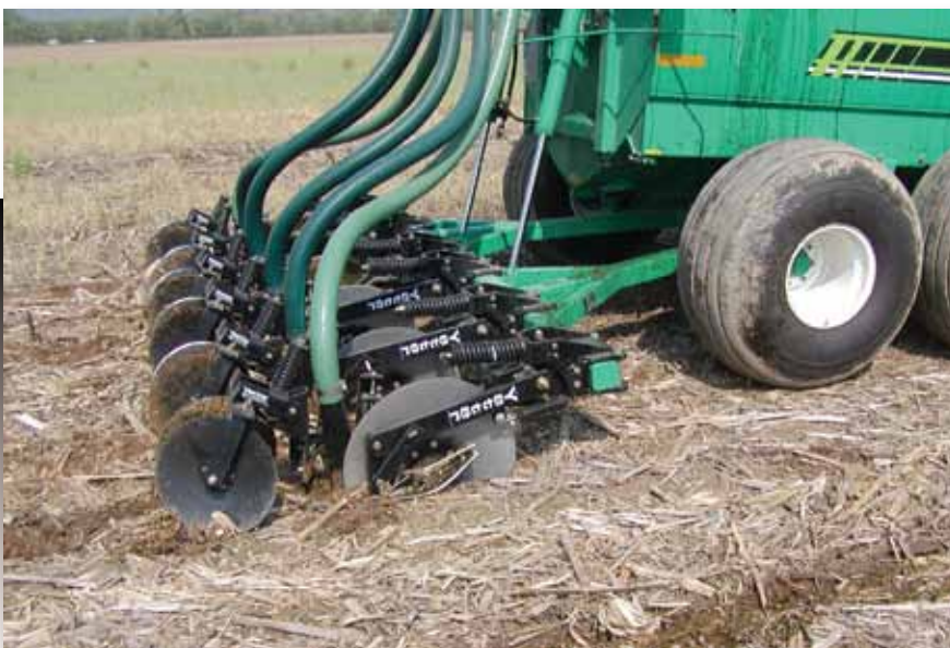
► Examples of novel manure application technologies currently available, including (clockwise) a disk injector system that is capable of injecting liquid manure to a depth of 15 cm; a chisel injector with sweeps, which includes a disk to cut surface residue; and an aerator set up to band liquid manure over the injection slots.
