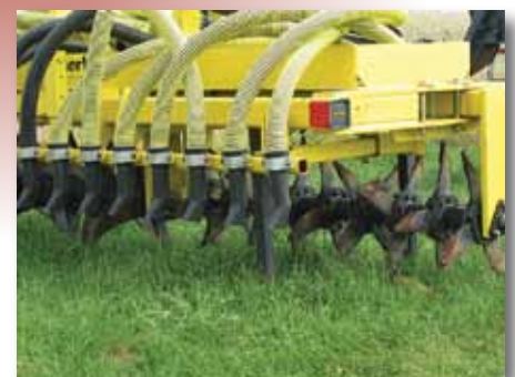
► Examples of novel manure application technologies currently available, including (clockwise) a disk injector system that is capable of injecting liquid manure to a depth of 15 cm; a chisel injector with sweeps, which includes a disk to cut surface residue; and an aerator set up to band liquid manure over the injection slots.
